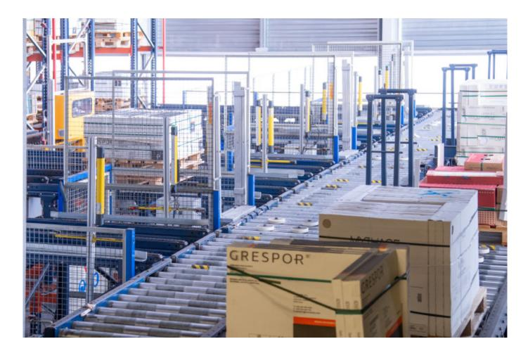
The warehouse management system distributes the goods in the AS/RS and assigns a specific location to each pallet. Easy WMS incorporates rules and algorithms that organize the items based on their characteristics and demand level. The aisles are divided into zones according
