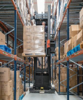
ing the products they need. To meet all of Elektro3's requirements, Mecalux has installed pallet racking with narrow aisles for three reasons: its adaptability to any type of load, weight, and volume; the direct access it offers to the products (facilitating goods handling and order picking); and its optimization of space.
