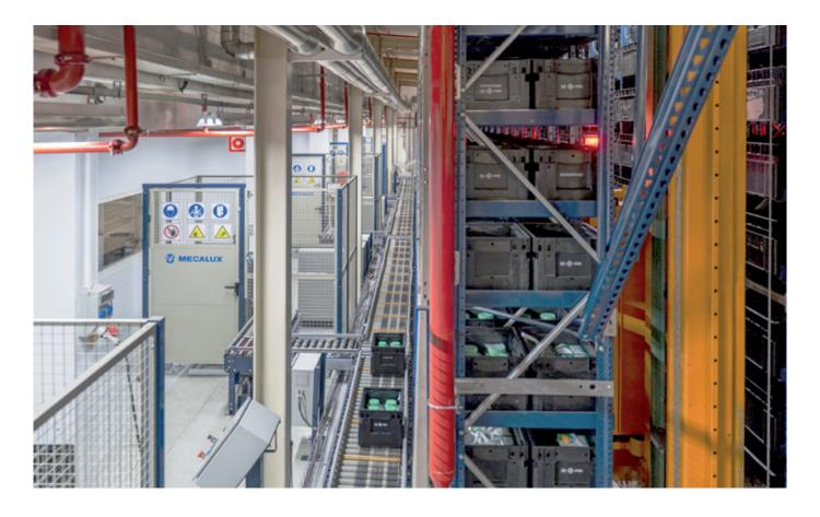
A total of nine lifts have been installed to link the center's two floors, separated by 14.7' in height. Seven of them connect the production lines to the AS/RS, while the other two bring the goods down to the lower floor, which houses the load preparation and dispatch areas.
