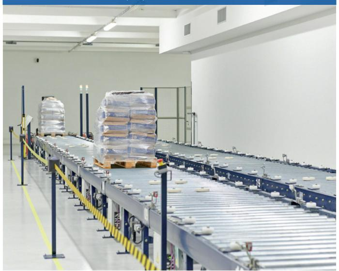
Vibar Nord, a producer of over 5,500 tons of food and dietary products a year, has opted for robotics in its new warehouse in Gera Lario, northern Italy. Mecalux has automated the connection between the production plant and dispatch area via a dual conveyor line and a pallet lift that automatically join the two zones. Mecalux has also implemented two earthquake-proof storage systems: Movirack mobile pallet racking and pallet racks, which have increased warehousing capacity by 70%.
