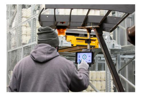
proposed the Interlake Mecalux Pallet Shuttle system and we agreed that it would work for our operations," Ramirez says. The high-density, semi-automated system uses a shuttle powered by an electric motor that runs along rails inside a storage channel.
