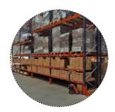
Picking locations On the lower levels of the pallet racks, M3 light-duty shelving and carton flow storage for picking have been set up. These two solutions serve to manage boxes and are specially designed for picking.
