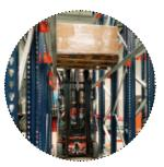
Drive-in racks With this compact system, operators use forklifts to enter the lanes with the goods raised above the level on which they will be deposited.
