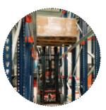
Drive-in racks With this compact system, operators use forklifts to enter the lanes with the goods raised above the level on which they will be deposited.
