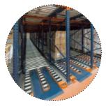
Live pallet racks These ensure optimal product turnover by applying the FIFO (first in, first out) method. Pallets are inserted into the loading aisle, slide by gravity to the other end and are ready for extraction.
