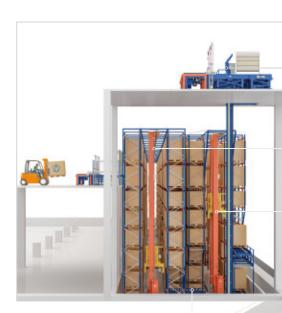
**Conveyors** Connect both storage aisles to transfer pallets.
