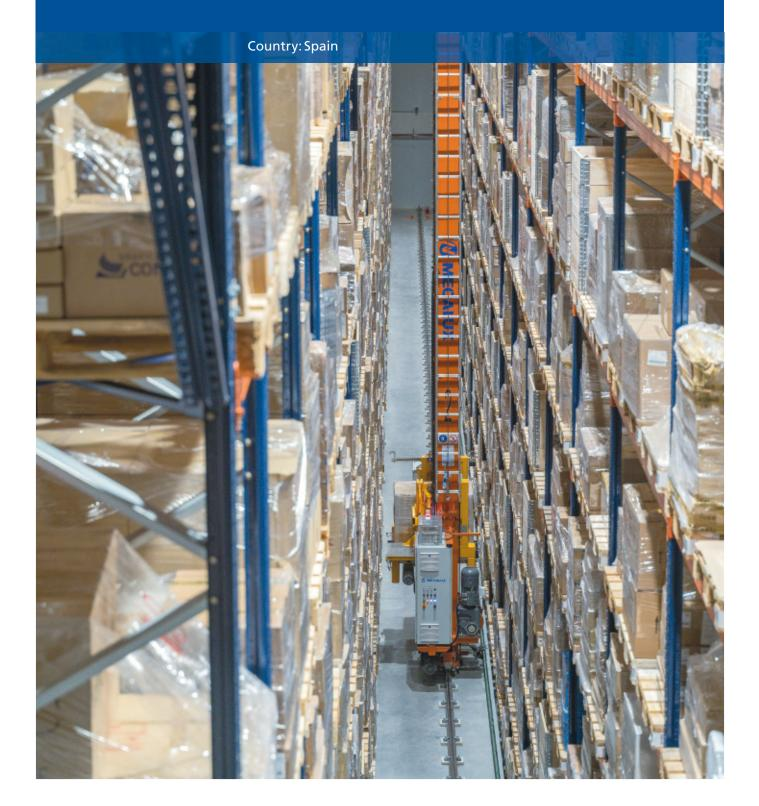
Cosmetics firm Natura Bissé has opened a new, completely personalized automated warehouse in Barcelona, Spain, where it has centralized all its goods previously outsourced to a logistics provider. Formed by merely two aisles storing 2,200 SKUs, this facility connected with production has been built in an 86-foot-deep pit. Mecalux has also implemented its Easy WMS warehouse management system to control product traceability in real time.
