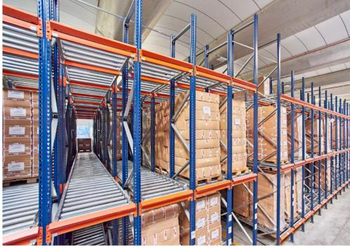
racks comprise three-level-high lanes. This solution reduces the number of aisles in the interest of maximizing space and, as a result, increases storage space.
