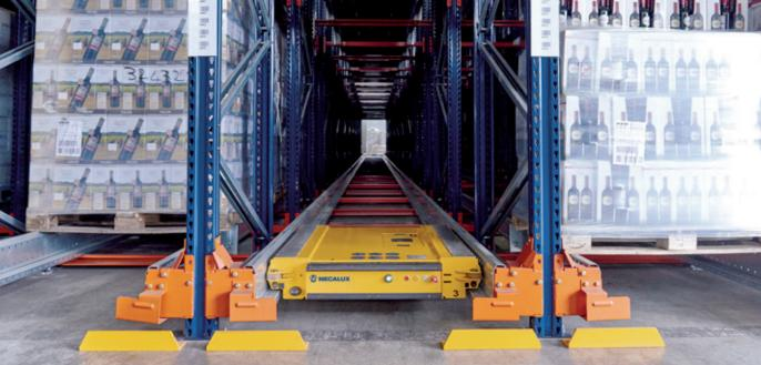
The Italian logistics operator Genta S.n.c. has a modern distribution center made up of high-density racks with the Pallet Shuttle system and pallet racks from Mecalux. The resulting storage capacity exceeds 7,000 pallets with alcoholic beverages. Space optimization and fast product inputs and outputs ensure quick deliveries to customers worldwide.
