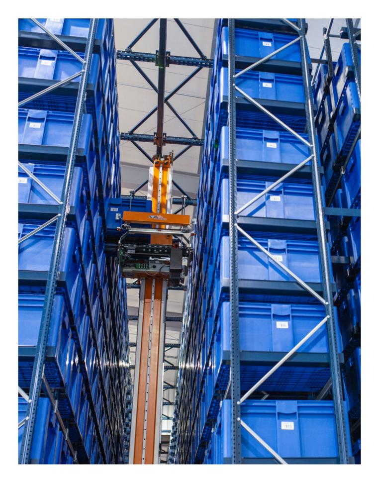
In an area of just over 3,875 ft<sup>2</sup>, the automated installation provides storage capacity for 11,904 boxes
