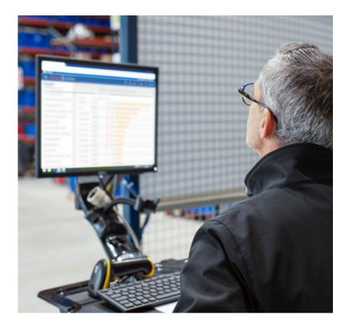
All operations in the automated installation for boxes are supervised by Easy WMS, Mecalux's warehouse management system. This software has a dual role: to update the inventory in real time and guide operators in picking tasks.
