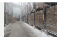
with the semi-automatic Pallet Shuttle system. This high-density storage system uses an electric shuttle to load and unload pallets inside storage channels. It was chosen based on the following factors:
