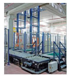
**Manual picking.** The manual picking stations are equipped with PTL (pick-to-light) devices that show the operators how to prepare each order, ensuring efficient and error-free picking.
