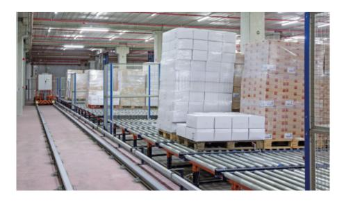
A complete preload is formed with pallets from three channels, so up to eight trucks can be left ready in advance. The transfer car, which can take two pallets at a time, sorts them into the corresponding channel according to the orders given by Easy WMS. The goods are grouped by route, vehicle, customer, delivery order and other characteristics, thus completing the entire sequencing process.
