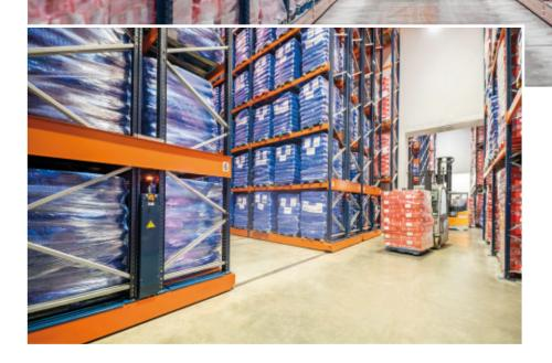
Mecalux has equipped the two new frozen storage units at Càrniques de Juià and Càrniques Celrà (companies that are part of the Olot Meats Group) in Girona (Spain) with Movirack mobile racks. This high-density system is ideal for frozen storage units. Its advantages: making the most of the available surface area and reducing energy consumption per pallet by optimizing storage unit volume. In total, the two warehouses manage more than 19,500 pallets.
