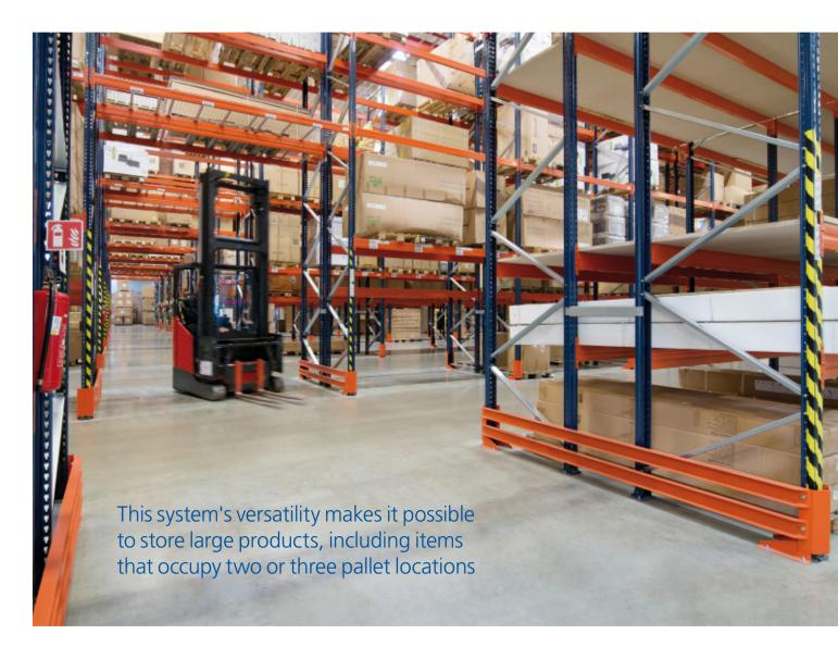
ble storage capacity: a total of 11,592 pallets. With such long aisleways, an underpass has been opened that crosses the racks transversely to ease the flow of operators and, in turn, use it as an emergency exit.
