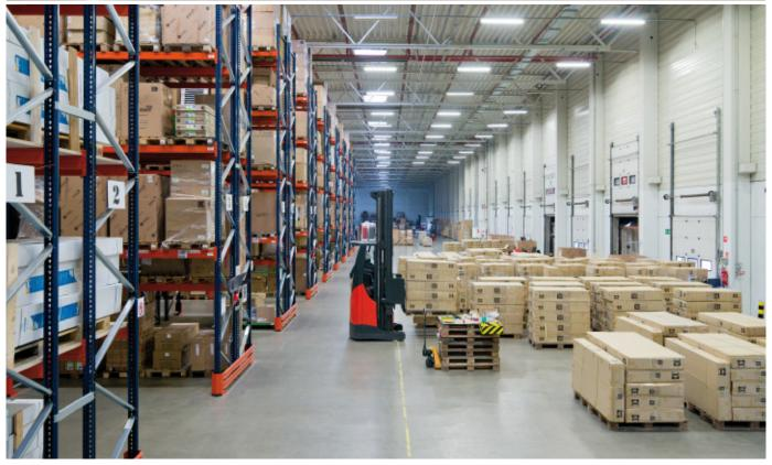
HSF e-commerce has equipped its logistics center in Sady (Poland) with 400' long Mecalux pallet racks that provide a storage capacity for 11,592 pallets. More than 10,000 SKUs of different volumes and dimensions are managed in this warehouse. The direct access to the racks quickens storage tasks and prep of 2,000 orders a day.
