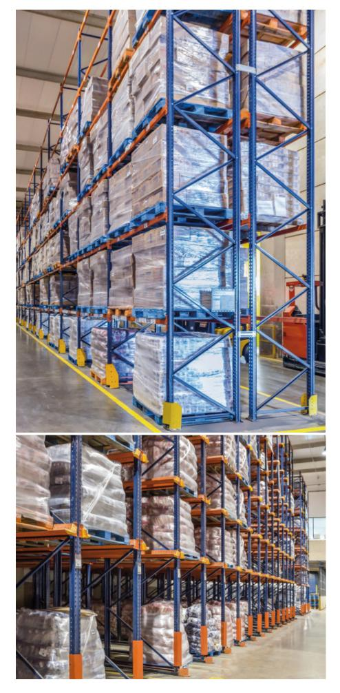
Operators, pushing reach trucks, enter the inner lanes with the load raised above the level where it is going to be deposited. On the floor, guide rails make it easier for forklifts to be centered and move safely inside lanes, minimizing accidental damage to the racking.
