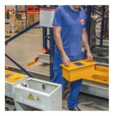
The operator sends movement orders to the Pallet Shuttle by means of a Wi-Fi connected tablet. It has a touch-screen interface and a very intuitive software that requires no special training to use. Each tablet can interact with all the shuttles in the warehouse, following a prioritization protocol. The battery charging system is easily accessible to operators. A spare insertable battery means the shuttles are always operational.
