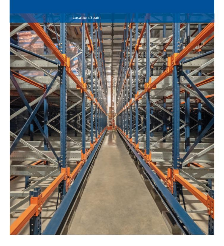
The Spanish meat company Cárnicas Chamberí has made giant leaps forward in its frozen storage logistics management in Toledo. Mecalux recently designed, built and commissioned an automated warehouse that holds close to 1,700 pallets for the business. The Pallet Shuttle was the system of choice — which operates via a stacker crane — because it speeds up the movement of goods and also cuts down on the power needed to create cold conditions.
