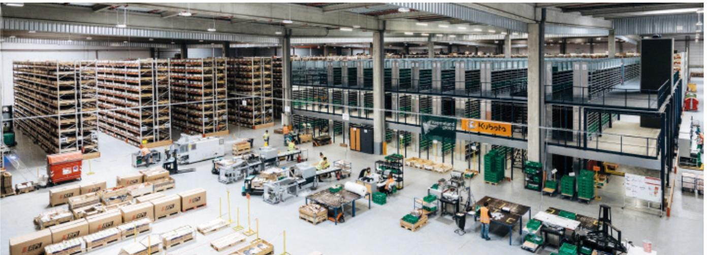
Kverneland Group, a farm equipment maker, runs a warehouse in Thionville, France, which it uses to distribute components and spare parts for its machines globally. Mecalux has equipped this warehousing installation with pallet racks, cantilever racks and shelving for picking to streamline picking of 550,000 orders per year.
