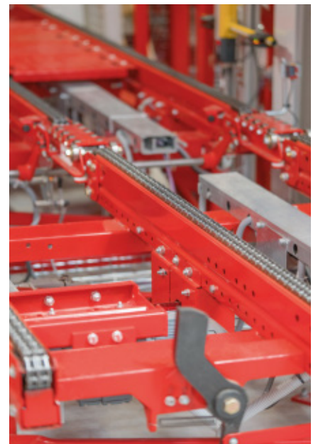
Hinged connectors bridge the gap between the pallets, ensuring pallet flows are continuous while the fire-resistant doors are open.
