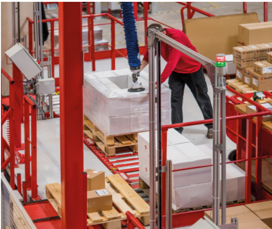
Hinged connectors bridge the gap between the pallets, ensuring pallet flows are continuous while the fire-resistant doors are open.
