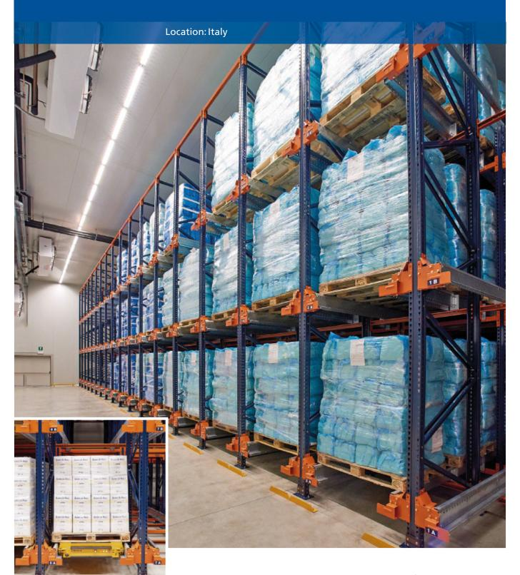
The butter producer Burro De Paoli has equipped both its frozen storage chambers in Italy with the semi-automatic Pallet Shuttle system. The installed storage solution boosts productivity, provides a 1,494 pallet capacity and minimizes the workforce.
