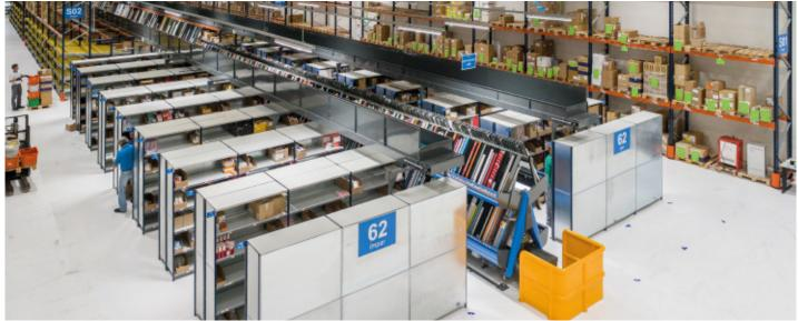
Operators remove items from inside the first box and place them in the corresponding carton compartment from the automatic box dispenser. The advantage of this storage system is stock reserves are housed on the same level, behind the first box, meaning product is always there for the taking.
