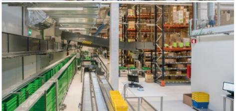
In the other two, dedicated to type B and C  $\,$ products, carton flow racks were installed with two attached conveyors and light-duty shelving units for the lower consumption boxes.
