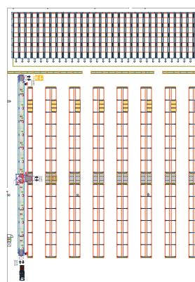
The first of these –in the middle of the circuit- coincides with the block of selective pallet racks and is where lower demand reserve products are sent.
