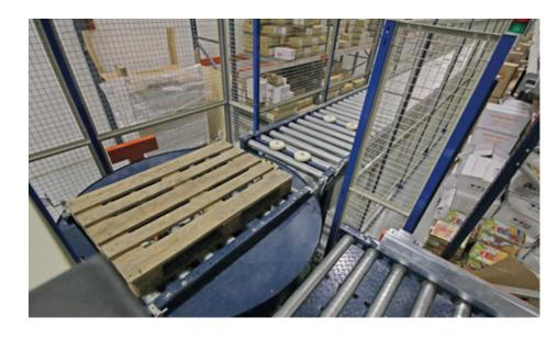
The conveyor at the Firat Food installation is 138' long and runs at a speed of 33 ft/min
