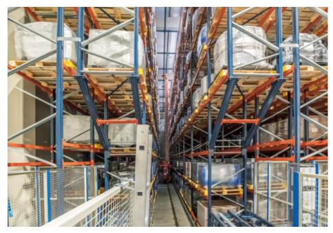
AS/RS stacker cranes have double-depth telescopic forks that help to deposit and extract loads from secondary locations on the racks
