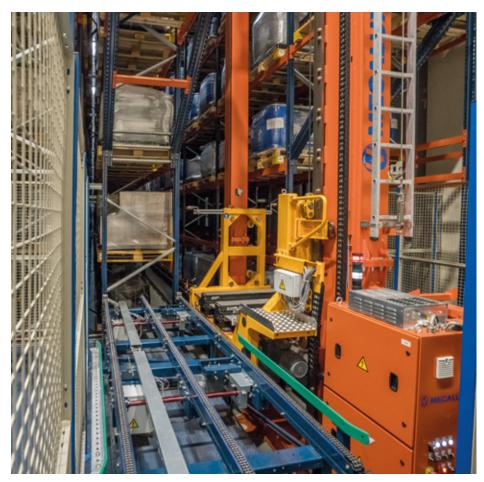
The goods leaving the warehouse repeat the same operation as when they enter, but in reverse. The pallet transfer car collects the pallets directly from the conveyor at the end of each aisle and moves them to the exit.
