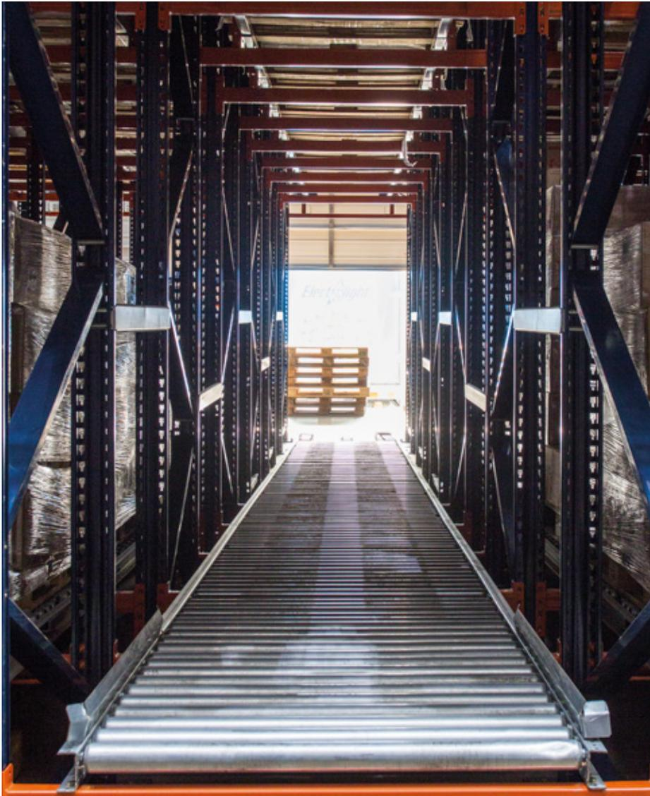
On the bottom level of the racks, pallet flow channels make product classification by order or route possible, and thus streamlined loading of distribution trucks
