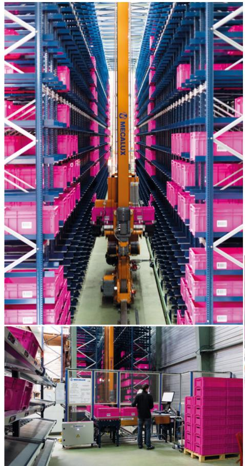
The 26' high warehouse consists of a single aisle with 98' long, double-depth racking. The 17 level racks contain a storage capacity of more than 4,000 boxes of 23''x 16" x 9"/13" and a maximum weight of 110 lbs each.
