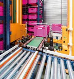
The miniload is an automated storage system for boxes that is an all-in-one installation with racks, stacker crane, conveyors and the warehouse management system. The solution implemented in the SCD Luisina warehouse is ideal for storing and picking according to the "goods-toperson" principle.
