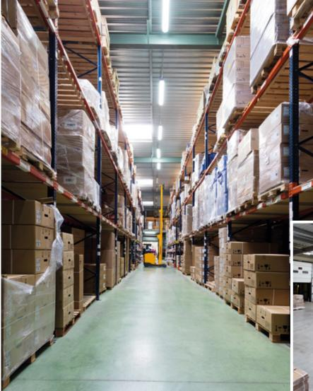
Parallel to the miniload installation, there is a 29' high pallet warehouse with an initial capacity of 2,700 pallets. At lower racking levels, bulkier goods and consumer goods are housed so that the operator can perform picking directly from the pallet. Reserves of each product are stored in upper spaces.
