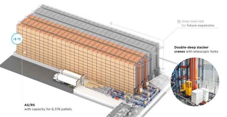
**Four live preload channels,** each with capacity for 17 pallets
