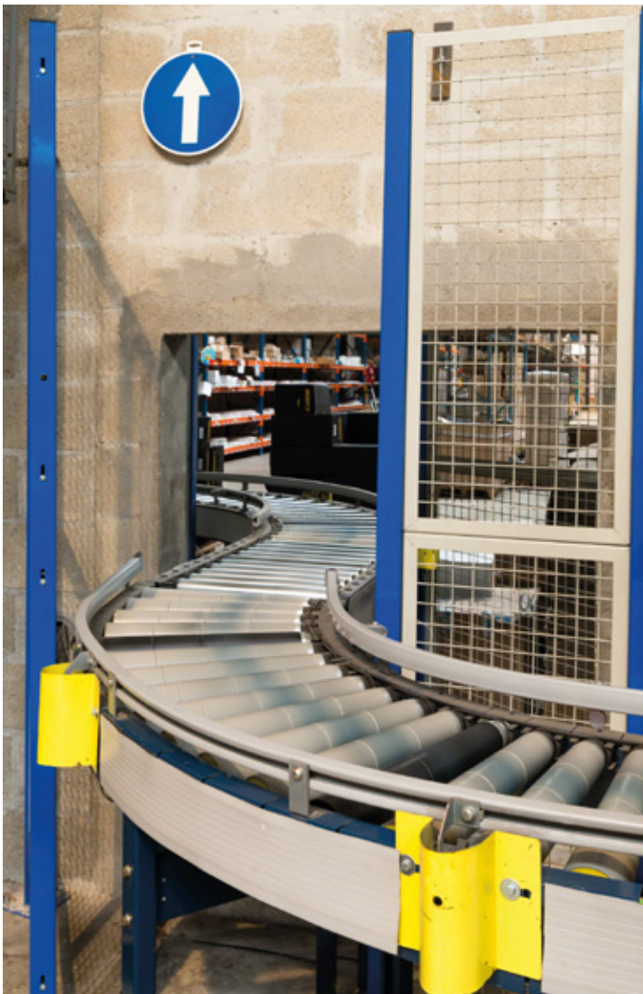
The hinged conveyor section can open so that operators may cross from one area to another
