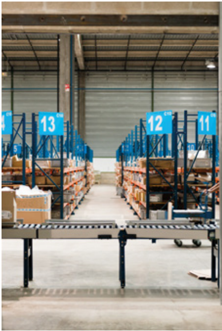
The hinged conveyor section can open so that operators may cross from one area to another
