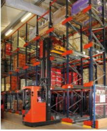
The Pallet Shuttle system permits faster handling of goods thanks to the automatic loading and unloading of pallets
