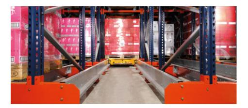
In addition, Mecalux offers the possibility of installing a positioning camera in the shuttle for the operator to view from the same tablet where and what the shuttle is doing at all times. Once the shuttle's battery runs out, the shuttle is automatically sent to the front of the channel, and the control tablet immediately notifies the operator that the battery is depleted. That is when it is moved to the battery charging station, set up to charge two shuttles at once.
