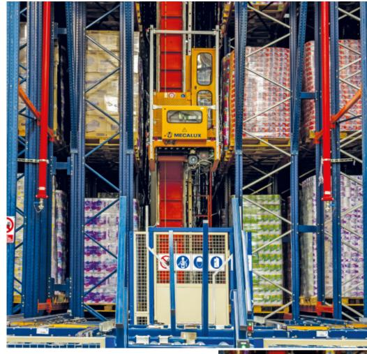
The installed automatic equipment ensures a high flow of goods per hour, to locate and remove pallets from the racking very quickly and without mistakes
