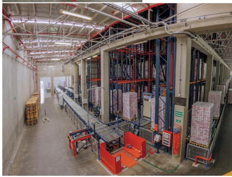
The recirculating conveyor circuit (double circuit) allows the management of inputs coming from production and from outside, as well as direct dispatches of palletized goods from the warehouse
