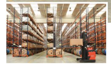
Trasgo's logistics center in Italy is sectored into four different areas to organize the goods of Enel — an important customer who distributes electricity — according to product characteristics and to comply with local fire regulations. Mecalux supplied pallet racking that offers a storage capacity of more than 20,200 pallets and ensures optimal management of any product.
