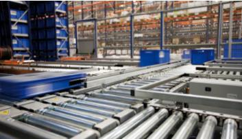
All processes related to picking begin in this area and are guided by the Mecalux Easy WMS warehouse management system. The first step is placing the boxes in the order prep positions located at the back and that also form part of the conveyor.
